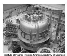
China's EAST tokamak, the first to use superconducting magnets, which enable it to confine the fusion plasma for a longer period of time.
